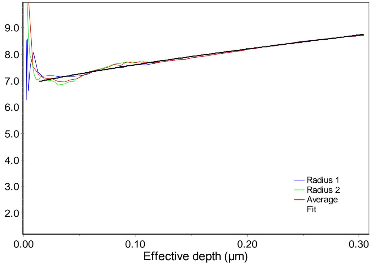
Radius function of indenter S10-6, nominal radius 10μm, obtained from elastic measurements on fused silica + sapphire
