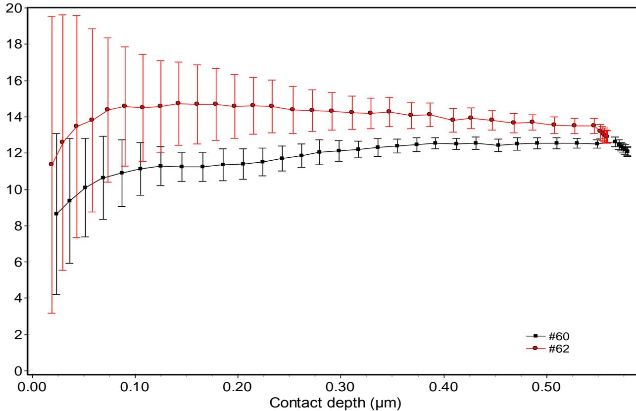
Indentation hardness as function of depth, measured with dynamic QCSM method of ASMEC
