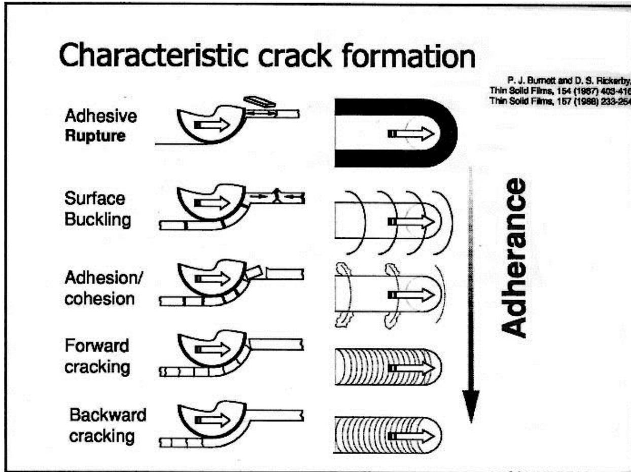
Failure modes for a standard scratch test with Rockwell C indenter
