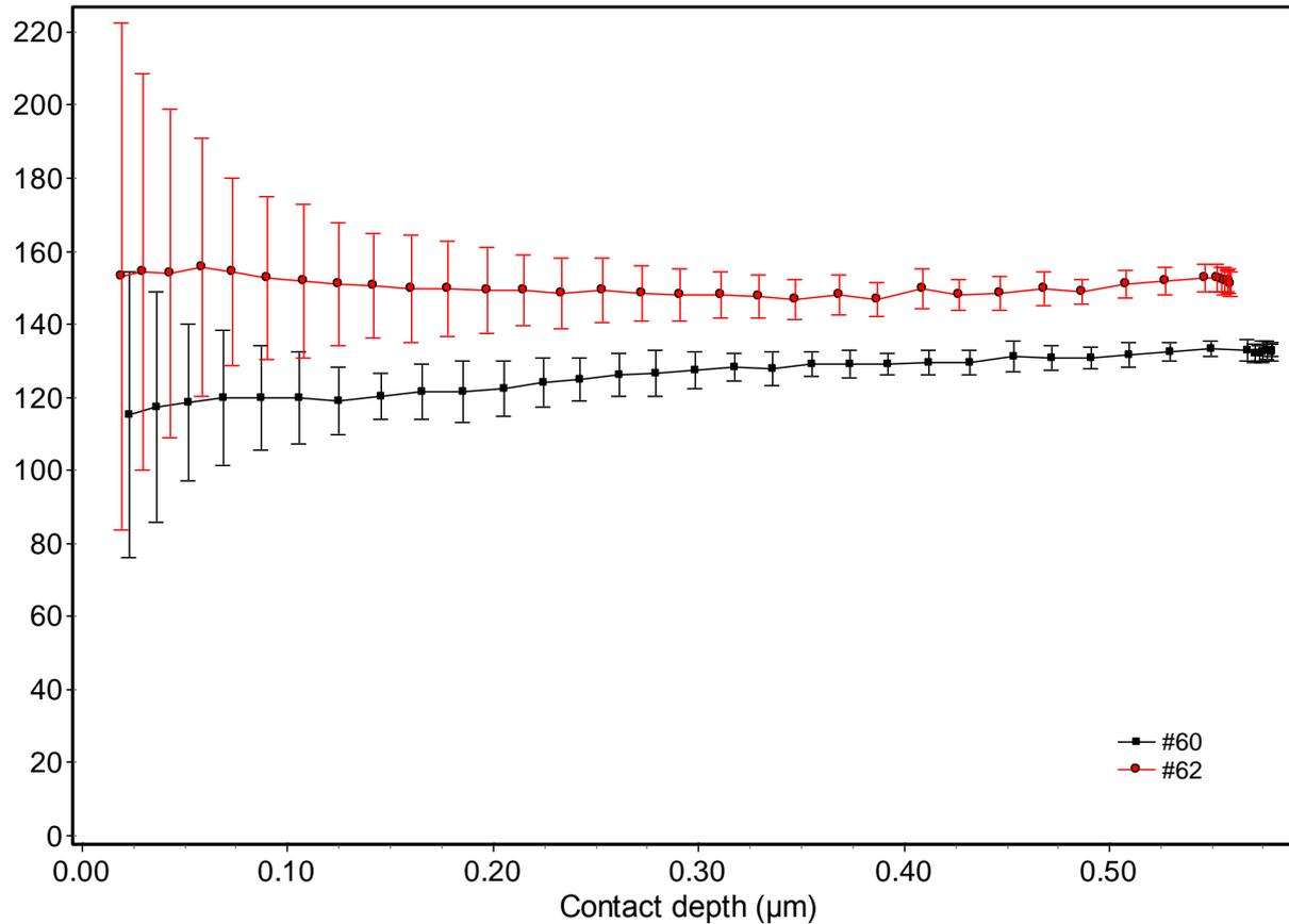
Indentation modulus as function of depth, measured with dynamic QCSM method of ASMEC
