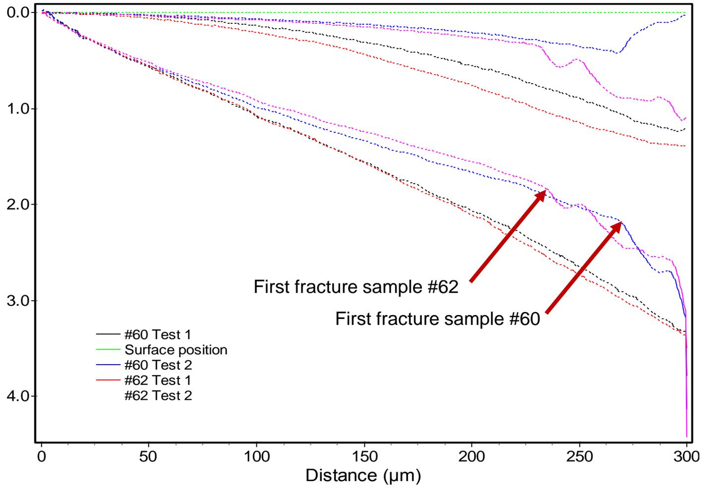
Comparison of depth under load and remaining depth from 1500mN tests on sample #60 and 62
