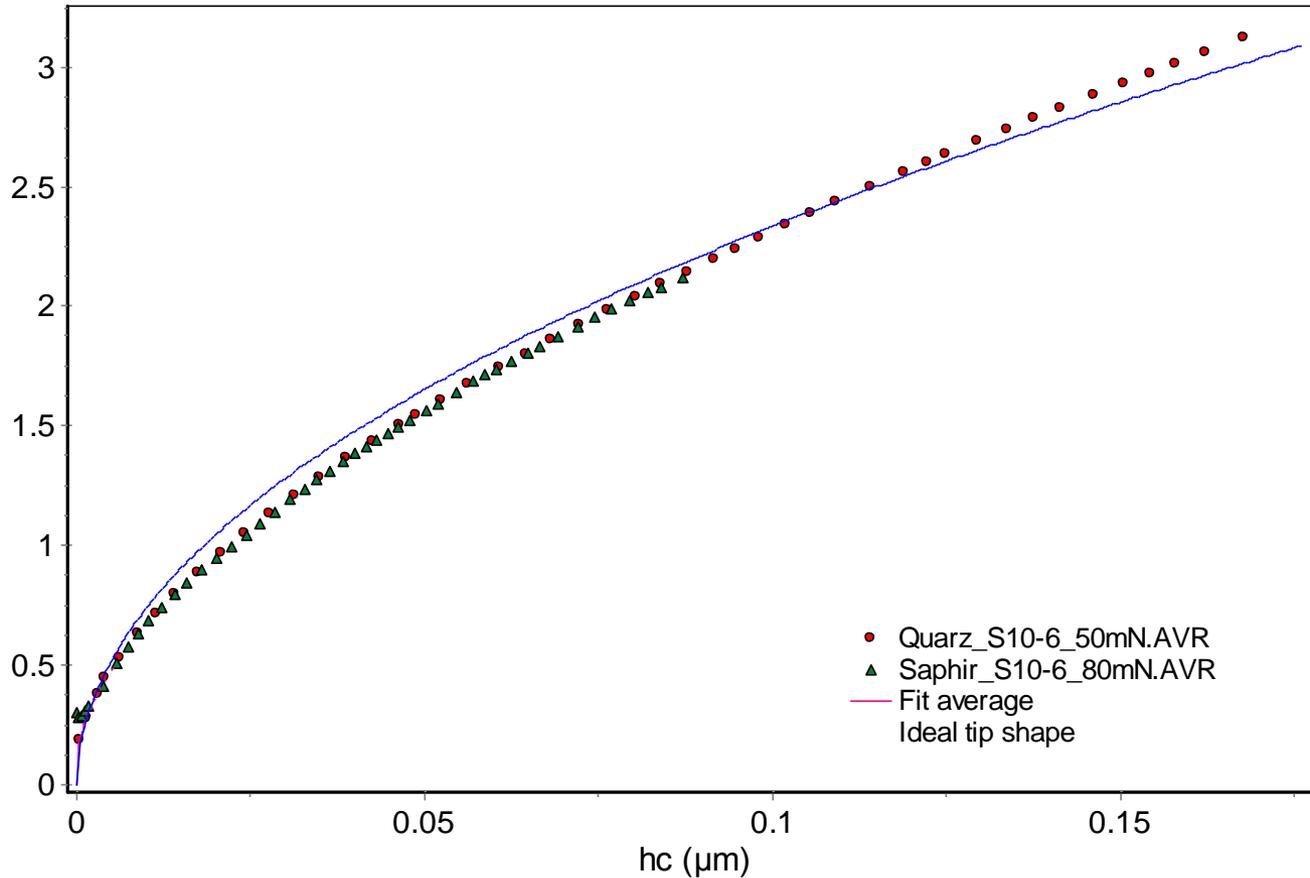
Area function of indenter S10-6, nominal radius  $10\mu\text{m}$ , obtained from elastic measurements on fused silica + sapphire
