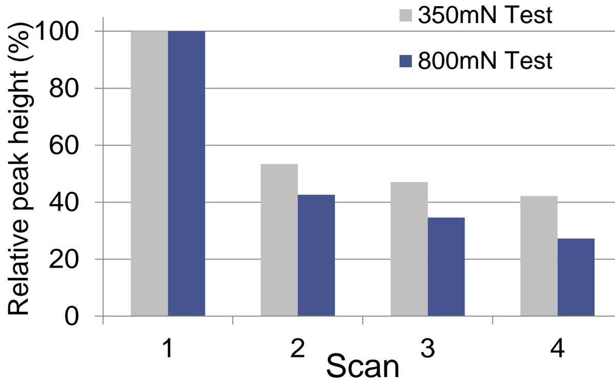
Reduction of the relative peak height of sample #60 during repeated loading
