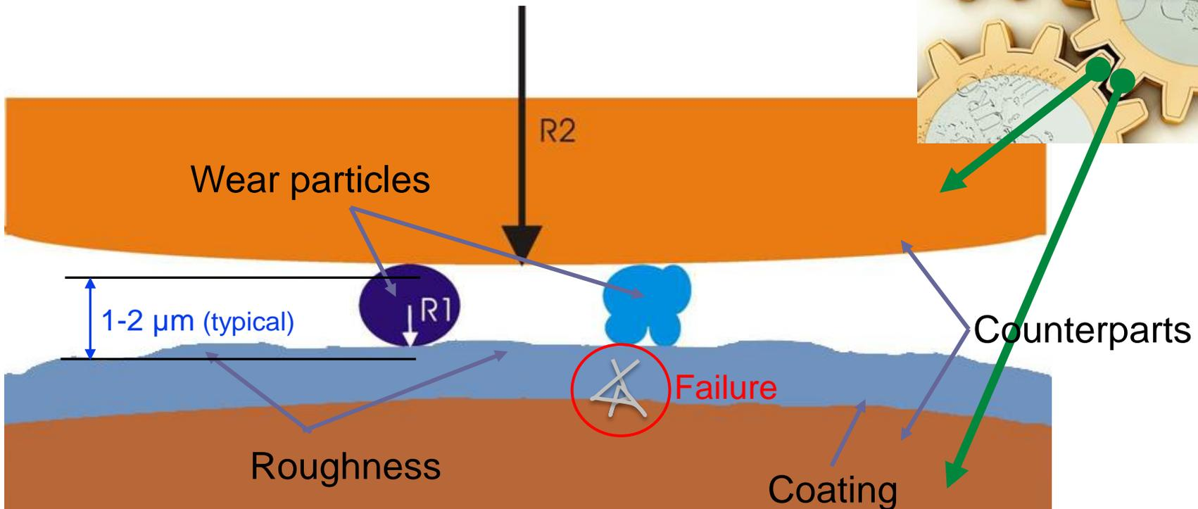
To understand the failure reasons one has to go down to the dimension of roughness and wear particles → This requires high resolution.
