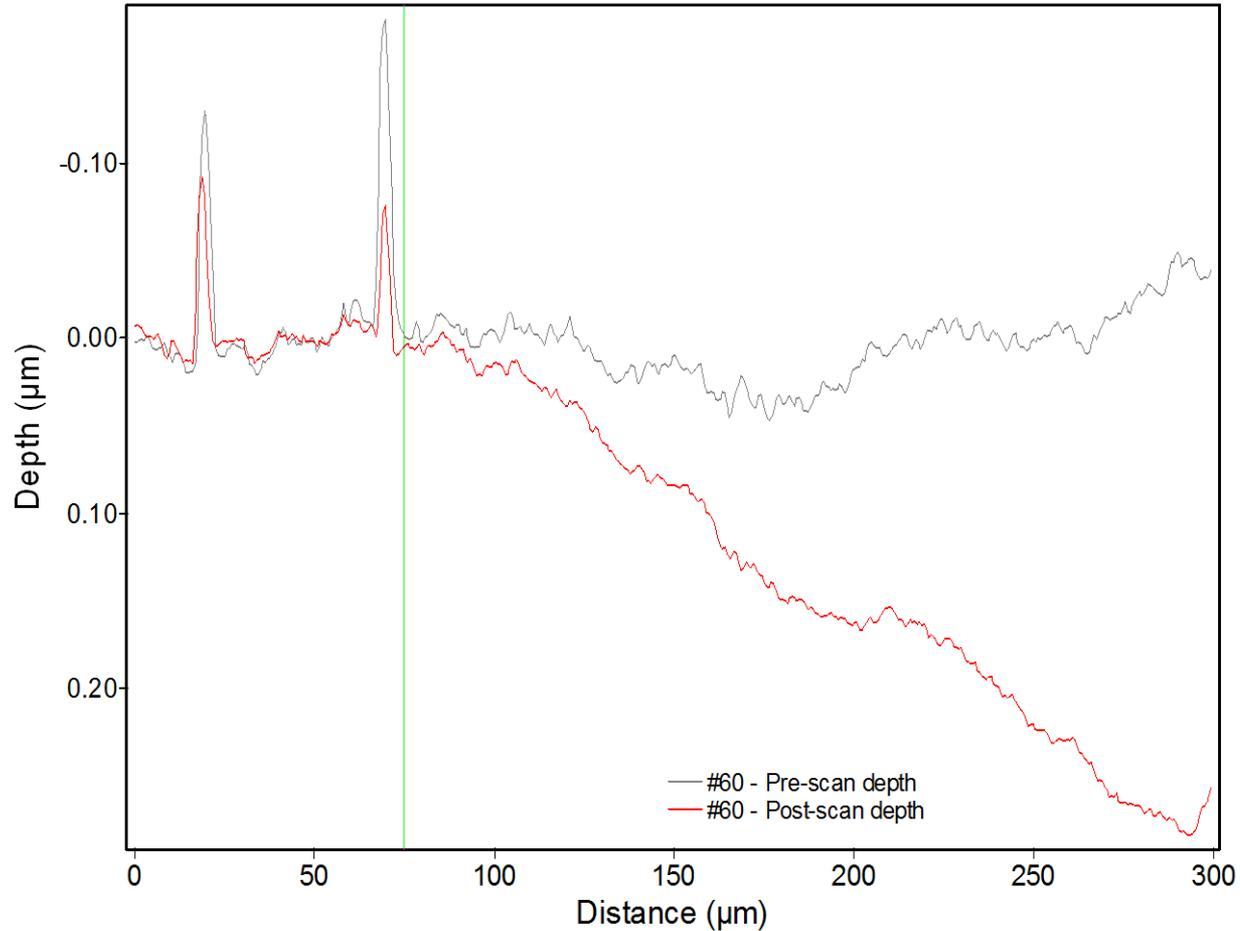
Comparison of surface position before and after test
