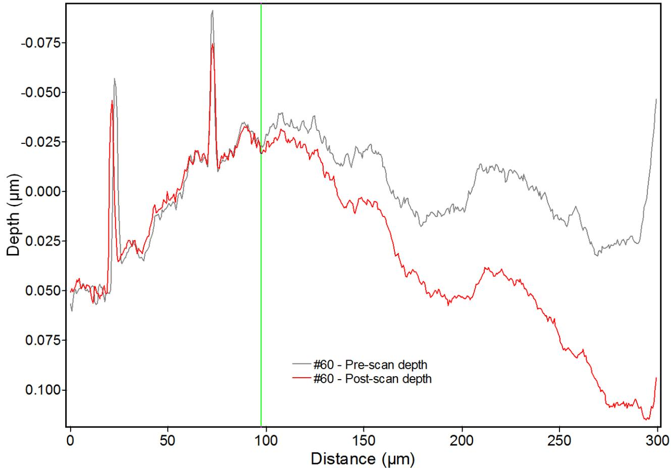
Comparison of surface position before and after test
