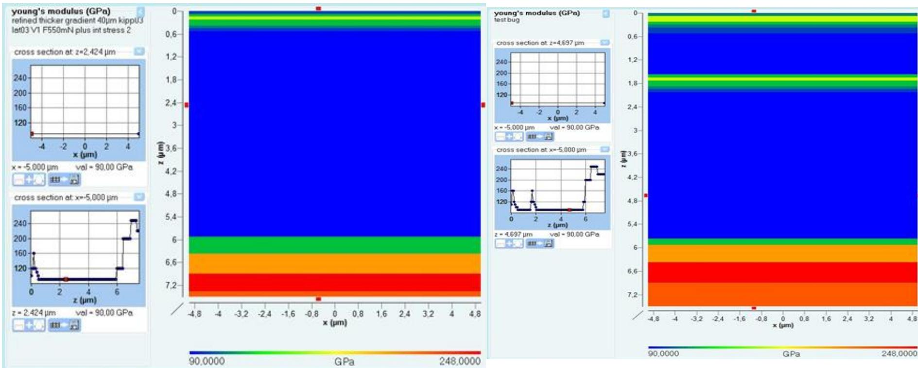
2 examples for an optimized layer structure for a certain roughness range and loading condition
