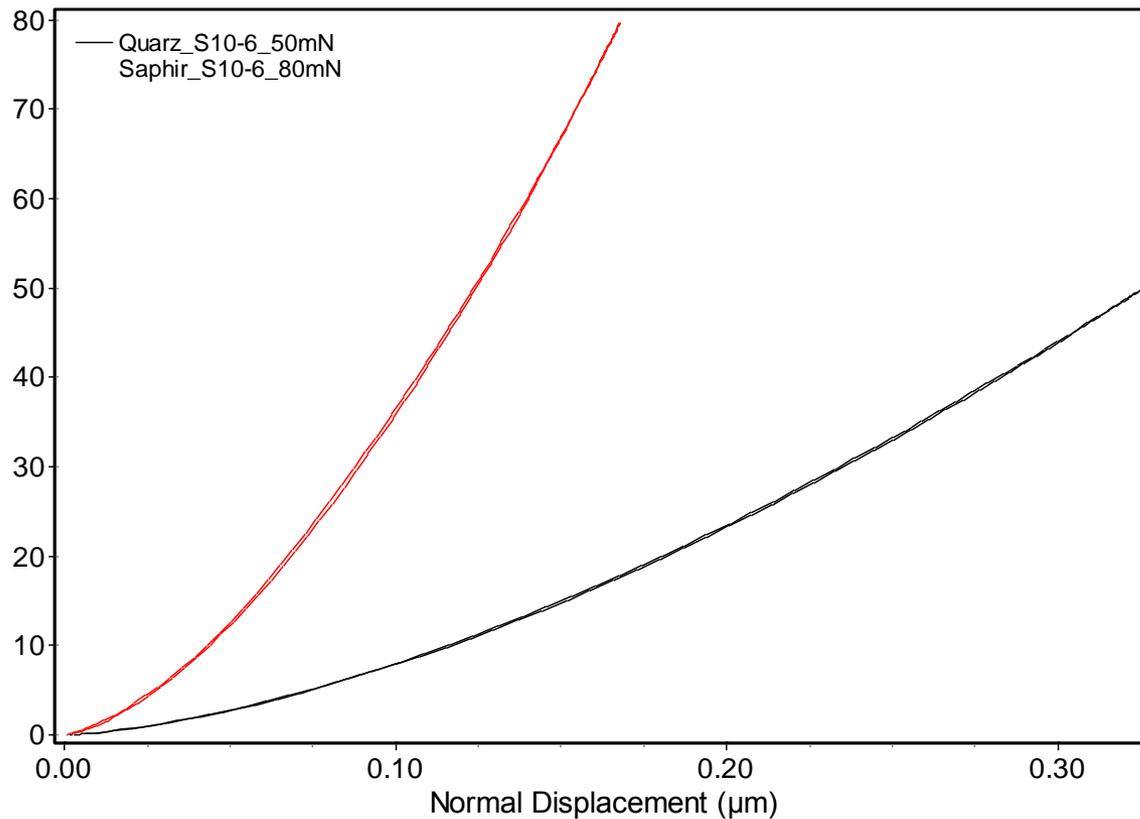
Fully elastic load-displacement curves, measured on fused silica + sapphire
