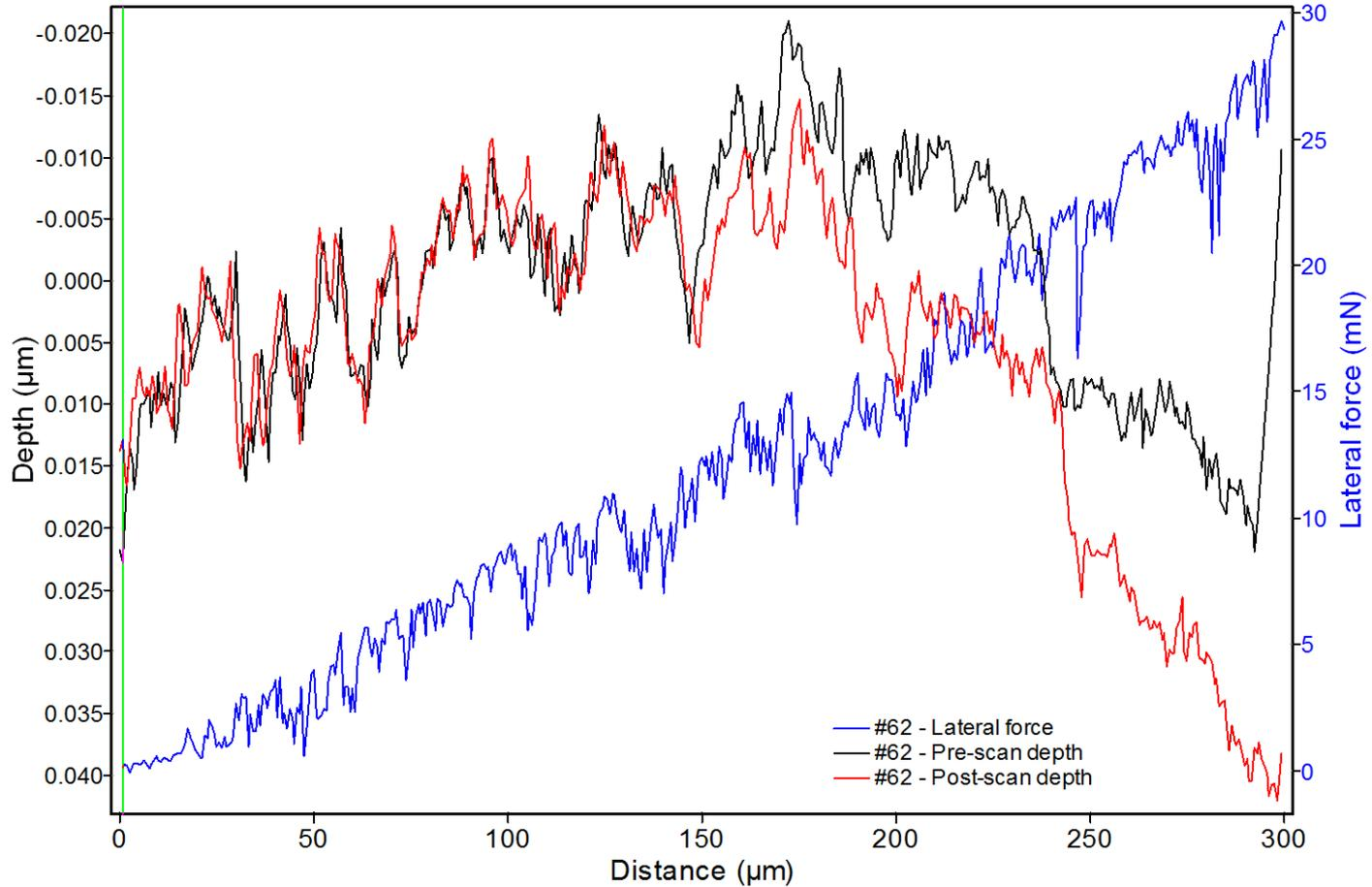
Comparison of surface position before and after test
