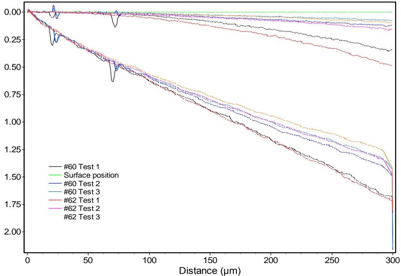
Comparison of depth under load and remaining depth from 800mN tests on sample #60 and #62
