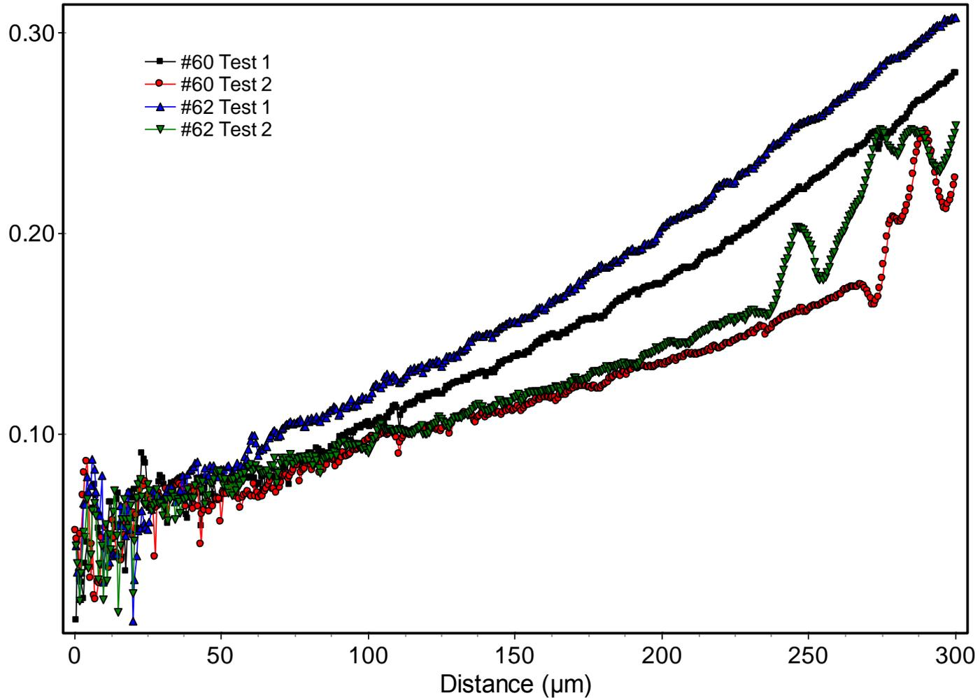
Comparison of friction coefficient from 1500mN tests on sample #60 and 62
