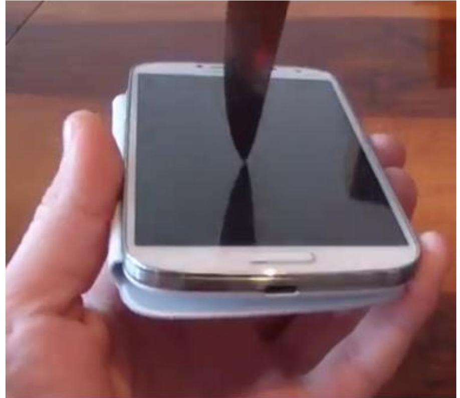
It depends on the sharpness of the counterpart if coatings can be damaged or not.
