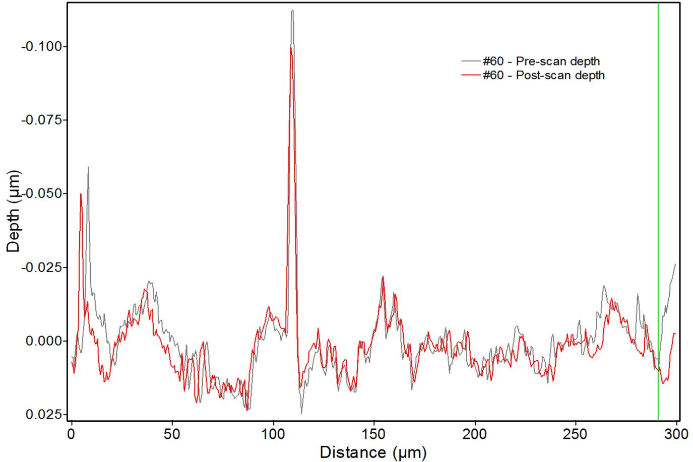
Comparison of surface position before and after test
