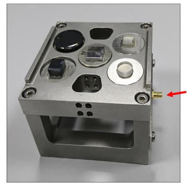
Connector for resistance measurement
