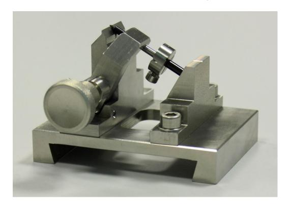
Sample holder for measurements at the tip of injection needles
